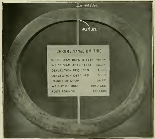
Chrome-Vanadium Driving Tire After a Drop Test.
